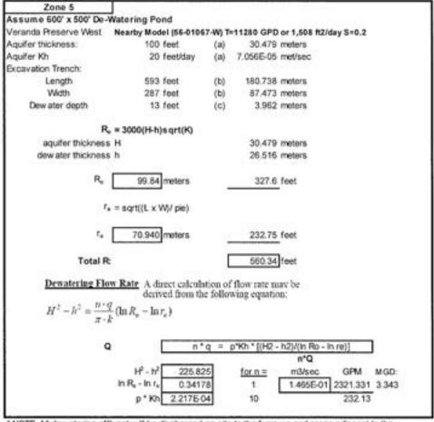
\* NOTE: All dew atering effluent will be discharged on-site to the furrows and areas adjacent to the proposed pond. Since dew atering effluent will be kept on-site this radius of influence is worst case scenario and the radius of the influence is highly unlikely to extend this far with on-site recharge.
